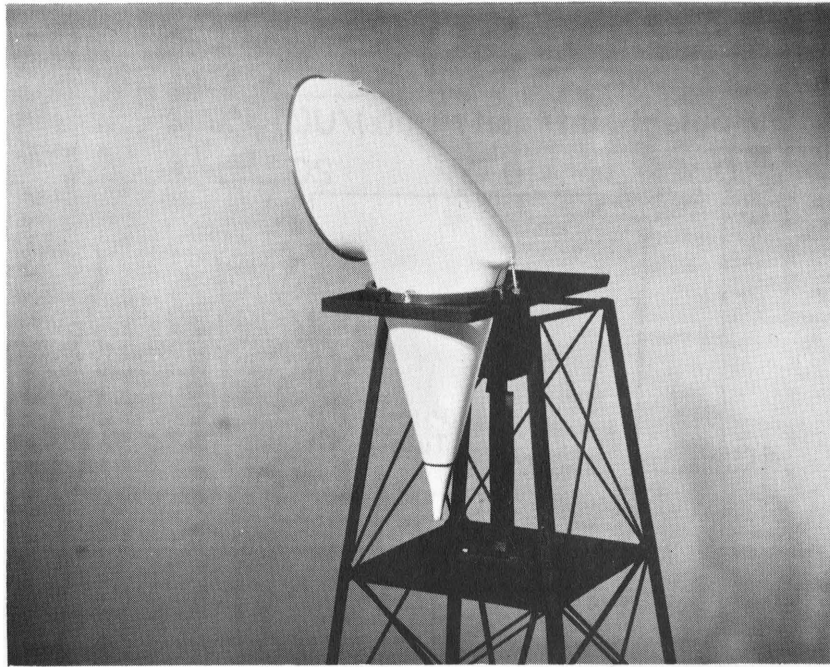
Fig. 6 "Gabriel" conical antenna horn mounted on a single horn platform
